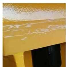
A close-up shot of an Easy-Qote corrosion-preventative patch
